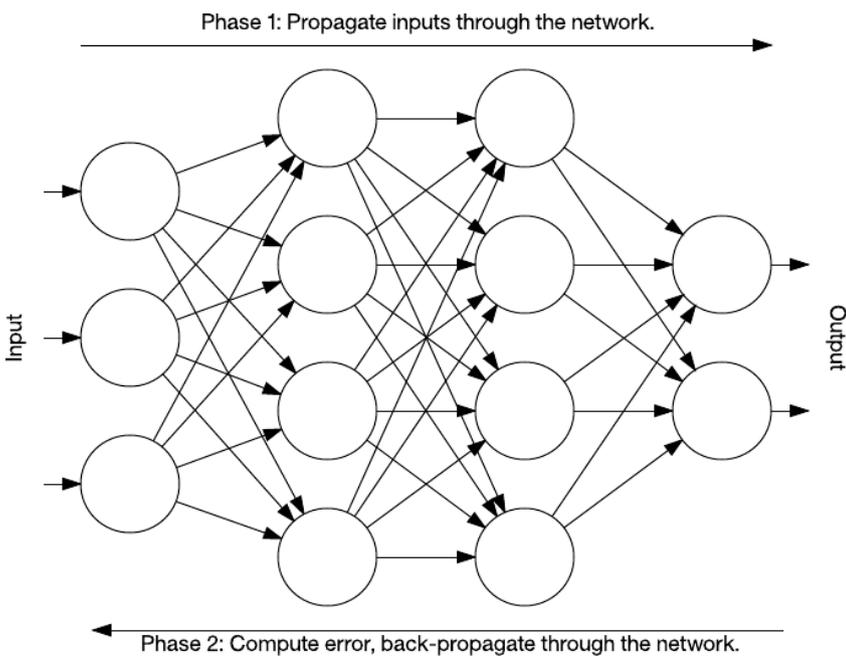
During training, intermediate layers of the network organize themselves to map portions of the input space to the output space. Backpropagation, through supervised learning, identifies an error in the input-to-output mapping, and then adjusts the weights accordingly (with a learning rate) to
