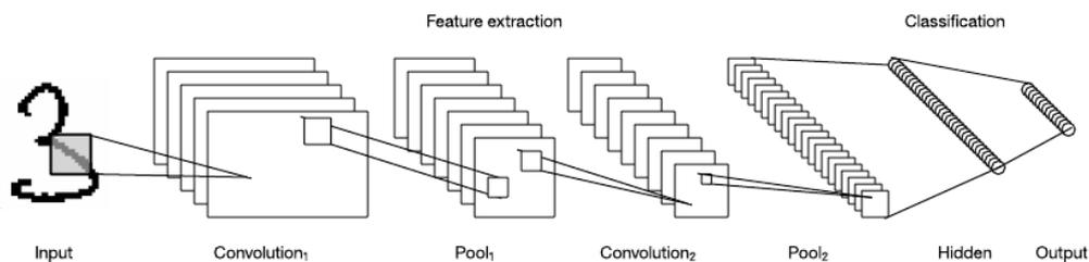
The use of deep layers of processing, convolutions, pooling, and a fully connected classification layer opened the door to various new applications of neural networks. In addition to image processing, the CNN has been successfully applied to video recognition and many tasks within natural language processing. CNNs have also been efficiently implemented within GPUs, greatly improving their performance.
