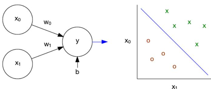
As a linear classifier, the perceptron was capable of linear separable problems. The key example of the limitations of the perceptron was its inability to learn an exclusive OR (XOR) function. Multilayer perceptrons solved this problem and paved the way for more complex algorithms, network topologies, and deep learning.
